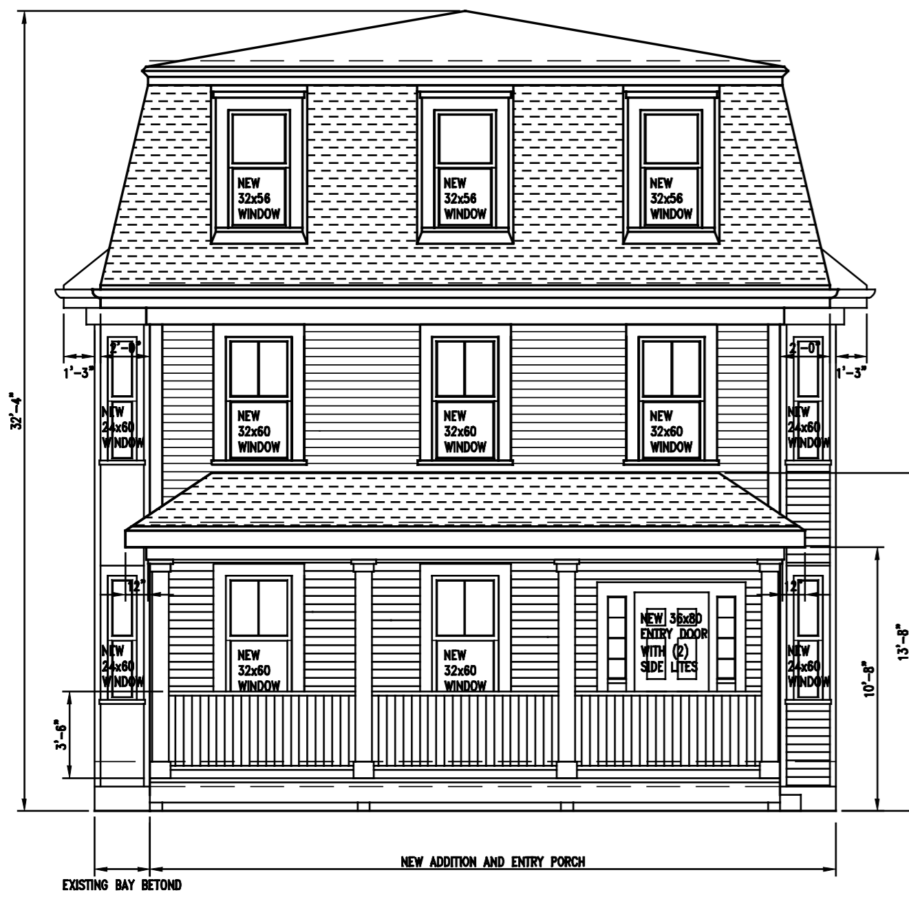
1 Front Elevation Scale: 3/16" = 1'-0"
