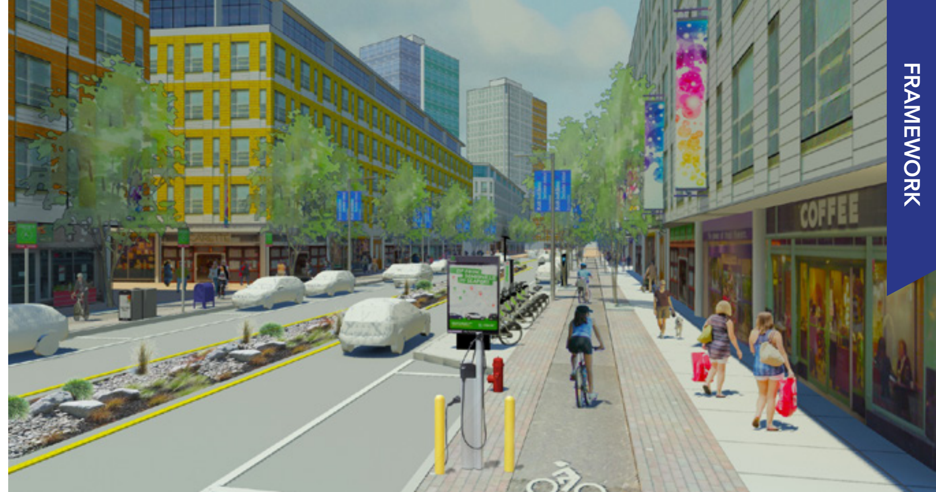
Figure 111. Opposite: Conceptual drawing of future Old Colony Ave that will include a designated bicycle lane and wider sidewalks
