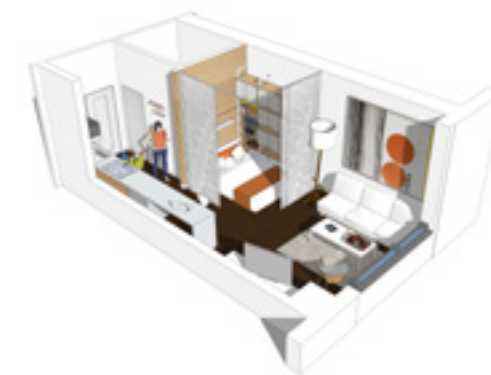
Figure 80. 3D compact unit design for 360 sf residential unit in Watermark, South Boston Waterfront
