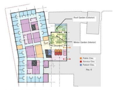
Floor Plan Level. 6 (7 & 8 Sim): Typical 30 Bed Unit
