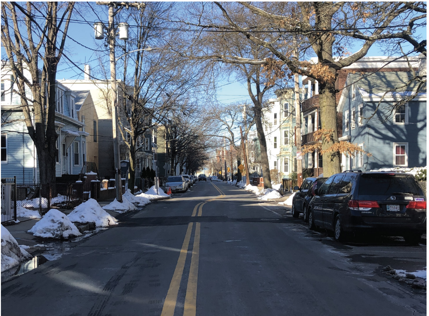
FIG 95 PHOTO | CHICANE FROM ALTERNATING PARKING ON HIGHLAND STREET IN SOMERVILLE.
