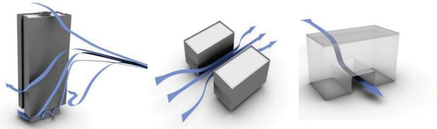
Image 4a – Downwashing Flow, 4b - Channeling Effect; 4c – Passage Acceleration
