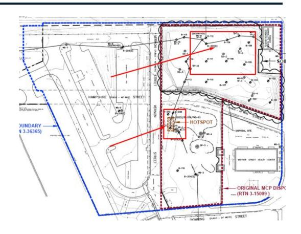
Our contractor, GEI, completed the soil testing. 24 bore holes were drilled at two main locations at the site.
