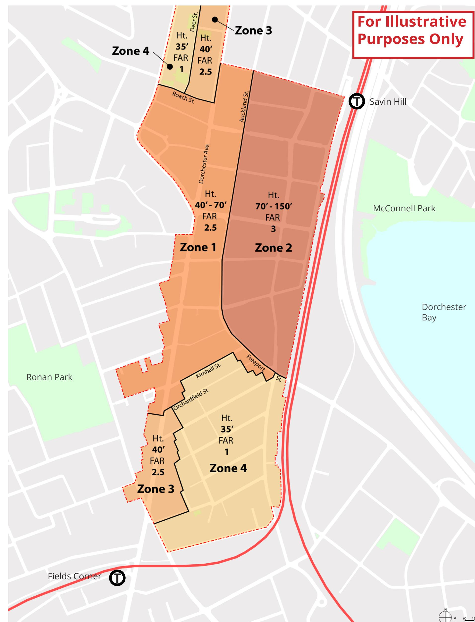
Height and floor area ratio diagram
