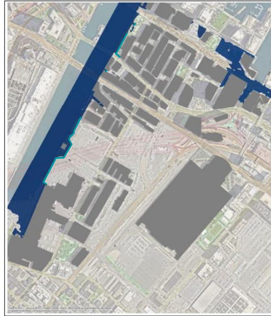
Flood extent during a 2030 100-year storm in existing conditions and with the proposed flood barriers in place
