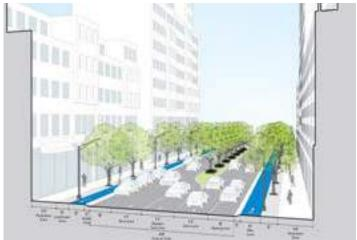
Main Street is transformed, eliminating multiple travel lanes and adding in a center median, cycle tracks and wider sidewalks.
