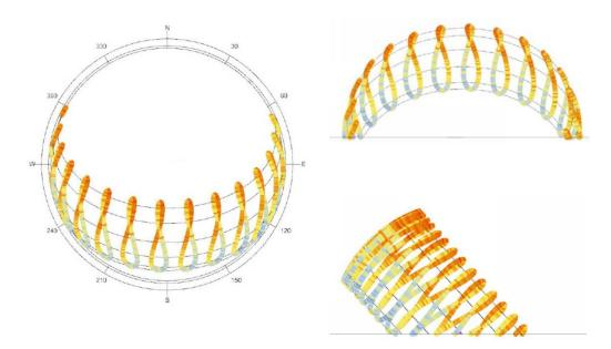
Image: Sun path diagrams for Boston, MA, plan view (left), view facing south (upper right) and view facing west (lower right).
