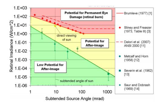
Image: Glare hazard plot illustrating the ocular impact as a function of retinal irradiance and subtended source angle.
