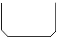
Chamfered edges or round corners perform better and reduce acceleration around building corners
