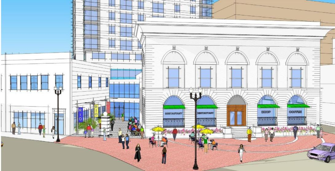
A two-story glazed atrium which links the two existing structures and the tower provides an accessible entrance to the Savings Building along with access to the office lobby and building management offices.
