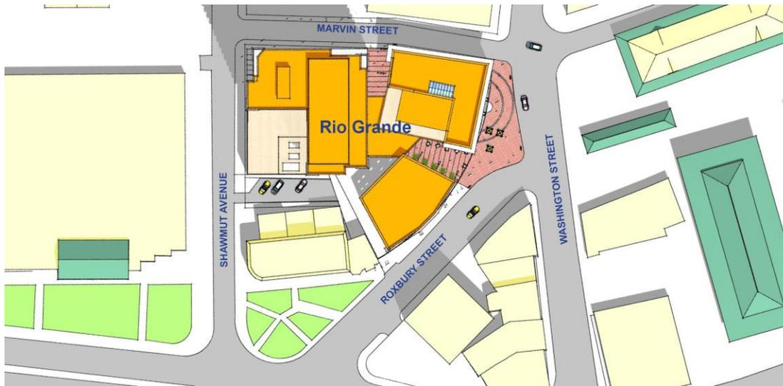
The Shawmut Avenue side of the Rio Grande Tower at the ground level is primarily purposed for loading and service functions. The north, west and south edges of the new tower are pro- posed to be constructed as close to the lot lines as possible and will likely require variances to current zoning
