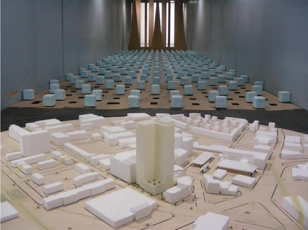
**Figure 2.30 Study Model Inside the GWE Wind Tunnel Looking Upwind**
