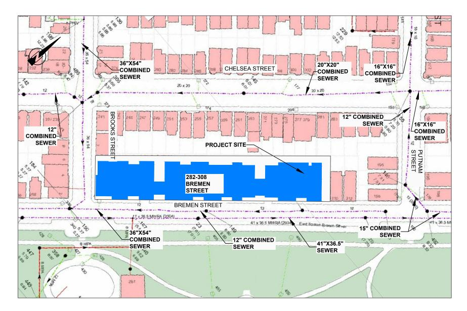
FIGURE 6-1 BWSC SEWER AND DRAIN SYSTEM MAP SCALE: 1"=120'±
