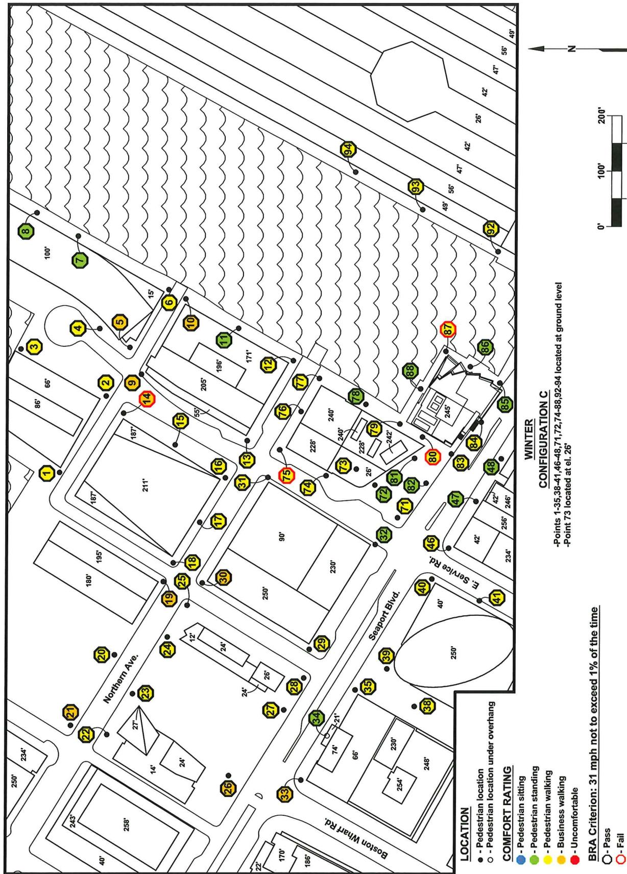
Figure 2g. Pedestrian wind speed measurement points with comfort/distress ratings – Winter.
