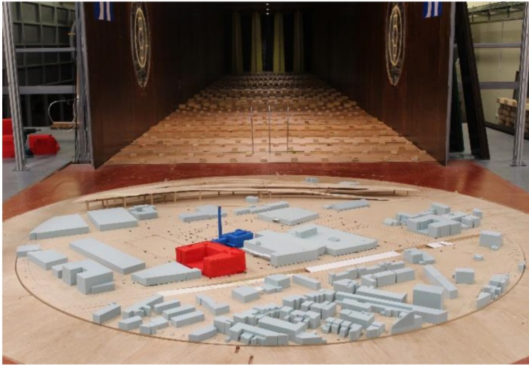
Image 1a: Wind Tunnel Study Model – No Build
