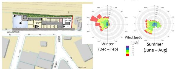
An analysis of the long-term wind data in the Boston area, shown in Figure 4, indicates that, on an annual basis, the most common wind directions are those between southwest and northwest. Winds from the east and east-southeast are also relatively common. Typically, winds are stronger in the winter and spring than those in the summer and fall.
