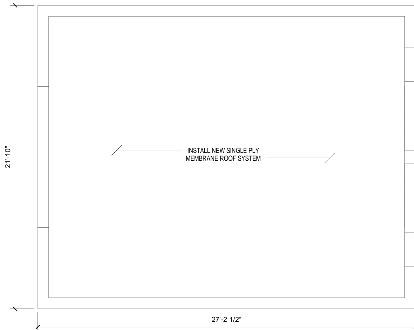
2 Garage Roof Plan - Proposed 1/4" = 1'-0"
