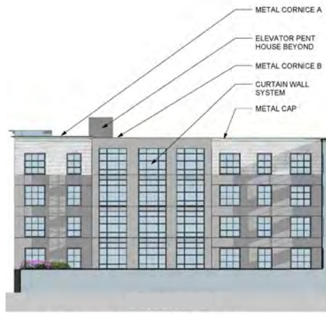
6 NORTHEAST COURTYARD ELEVATION 1" = 20'
