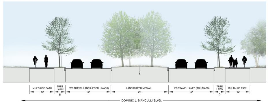
Section through Bianculli Boulevard near the intersection with Morrissey Boulevard. The diagram shows two 12' multi-use paths. Alternatively, these could be separate 7' bicycle paths with 5' sidewalks.
