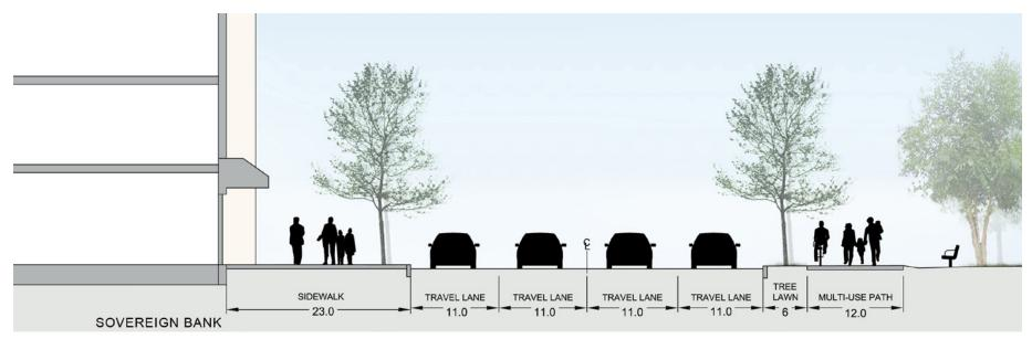
Section through New Street illustrating wide sidewalks, two travel lanes in each direction, and a 12' two-way multi-use path on the right (new buildings on Sovereign Bank parcel at left and Boston College High School on right). Alternatively, the road could be designed with two 7' one-way bike paths with separate sidewalks. The dotted line in the diagram above illustrates an alternative alignment that avoids the existing buildings on the Sovereign Bank parcels.
