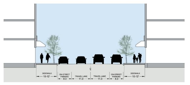
Section of typical two-way internal street with 7' sidewalks, street trees and on-street parking.
