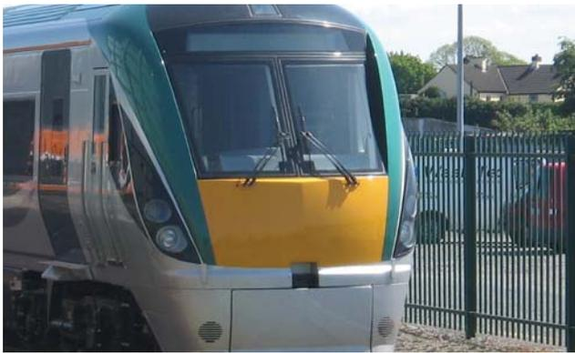
An example of a diesel multiple unit (DMU) train
