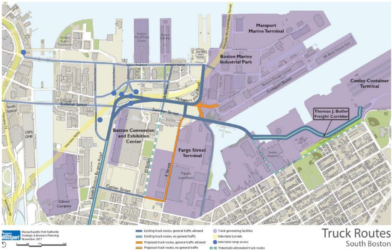
Figure 25: Existing (as of November 2017) and proposed truck routes in the South Boston Waterfront (source: Massport)
