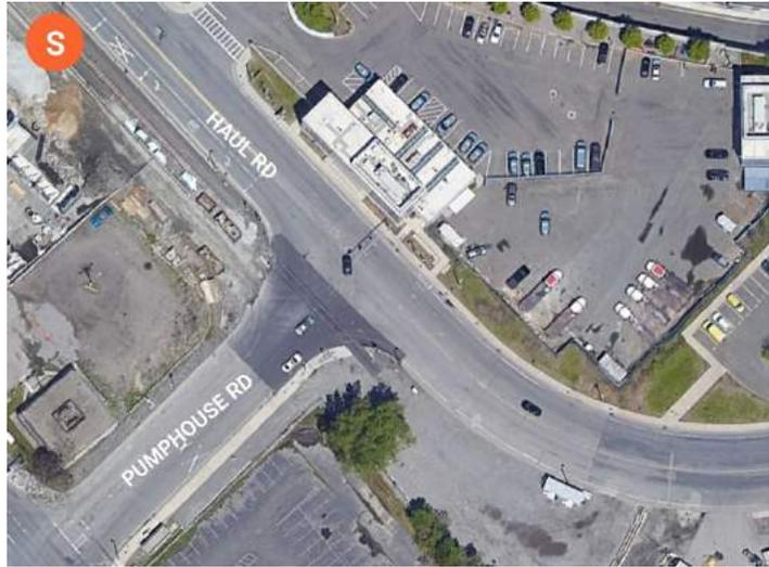
Crosswalks are present along the Haul Road eastern approach but are significantly faded. Pumphouse Road does not feature sidewalks in the southbound direction and Haul Road does not feature sidewalks in the eastbound direction on either approach. Rail tracks (Track 61) run across the Pumphouse Road approach within the intersection.
