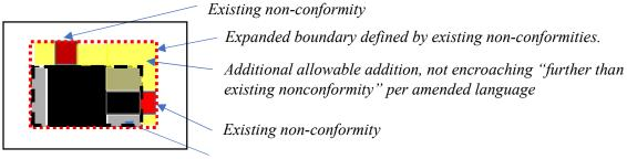
Allowable addition conforming to dimensional requirements
