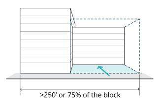
Figure 3: Buildings with extremely long facades in excess of 250 feet in length or 75% of a block (whichever is smaller) should use more and larger scale physical openings and setbacks
