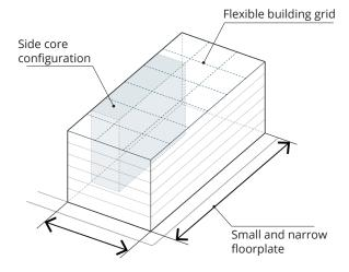
Figure 2: Designs that optimize the flexibility and future use opportunities of a building are encouraged. A smaller and narrower floorplate, adaptable building grid, and side-core configuration can create efficient and flexible layouts for a mix of uses.
