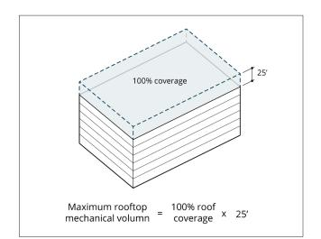
Figure 4: Rooftop mechanicals should be contained within a envelope limited in volume.
