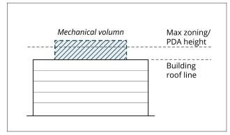
Figure 5: The volumetric limit to rooftop mechanicals generally applies to mechanical equipment located above the established building height in zoning. However, to encourage the integration of mechanical equipment into the building design, independent penthouse structures are calculated in their totality, and measured from the roof line regardless of the building height in zoning, as illustrated in example above.
