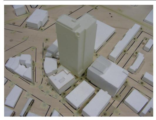
Figure 2.31 Study Model Inside the GWE Wind Tunnel Looking Upwind
