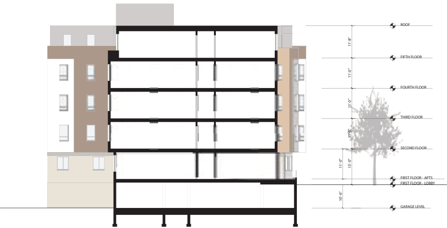
Five Story Apartment: Section Across Circulation Core
