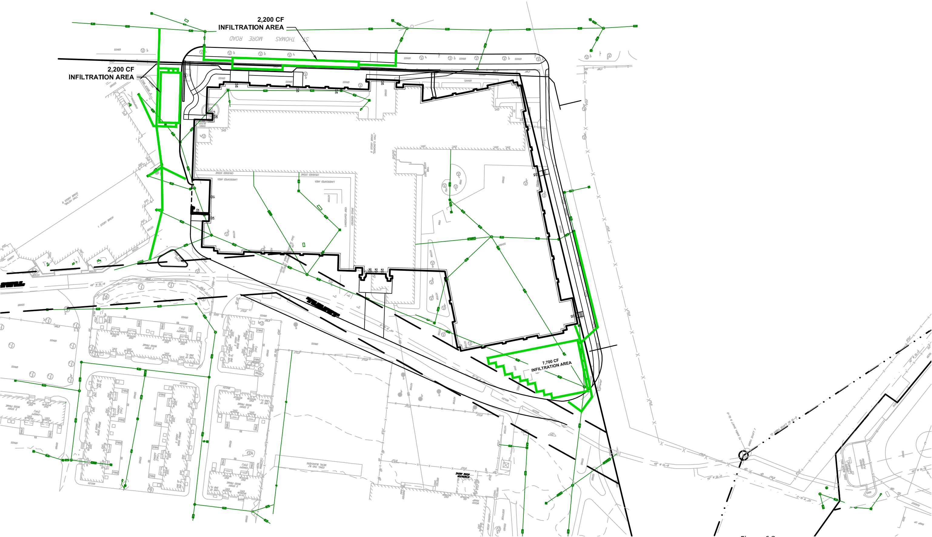
Figure 6.2 Proposed Stormwater Managment Improvements
