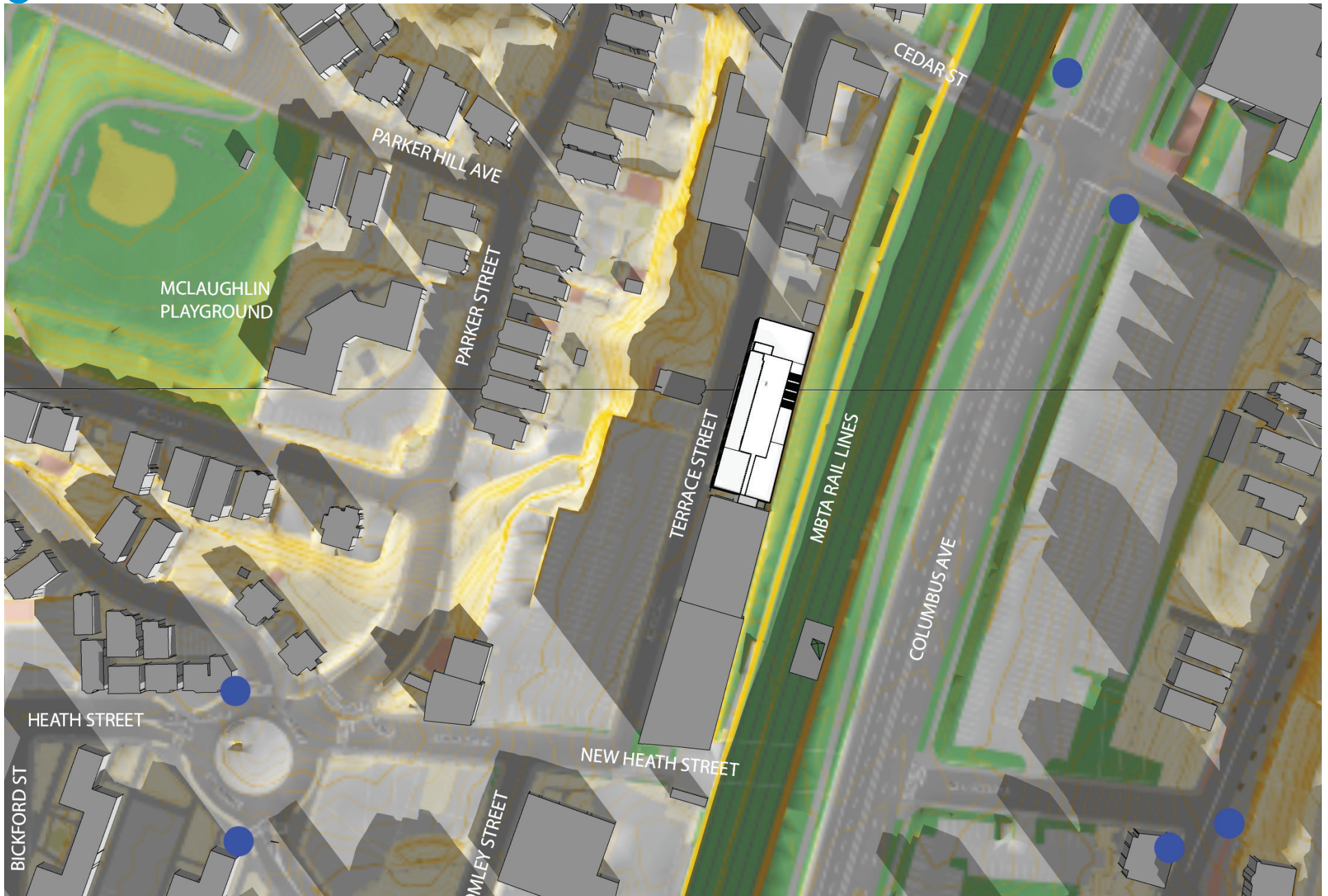
Figure 4.1-13 Shadow Study: December 21, 9am Alt 14.4 Azimuth 142.0
