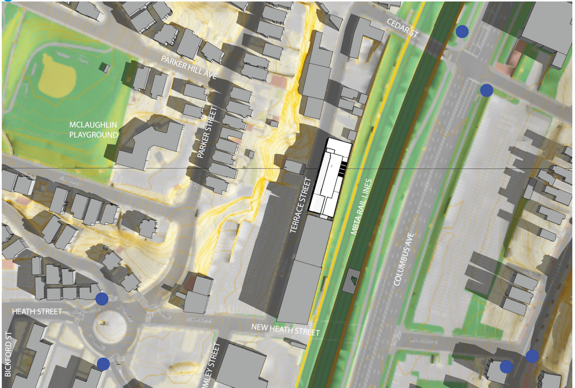
Figure 4.1-9 Shadow Study: September 21, 9am Alt 26.1 Azimuth 115.2
