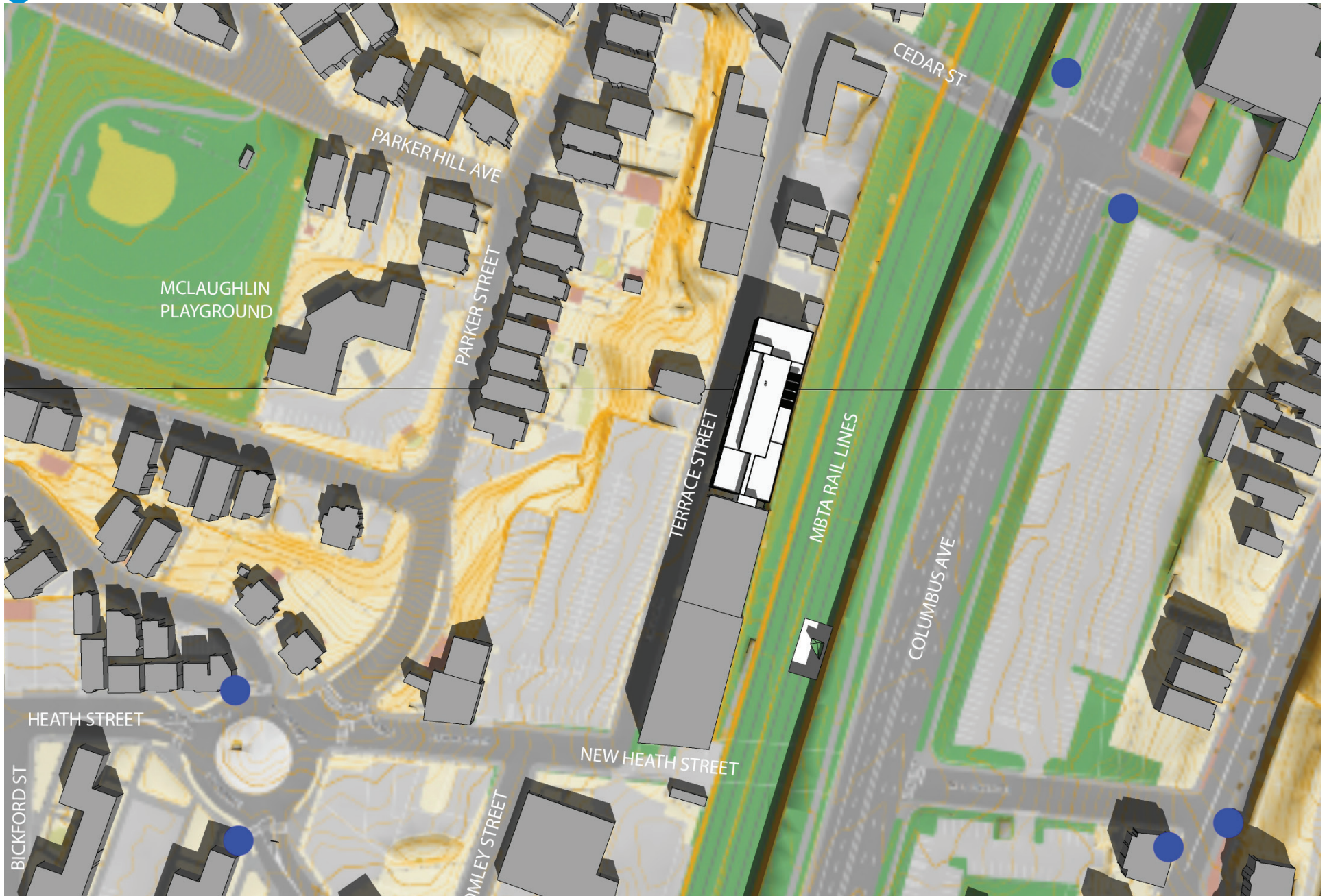
Figure 4.1-2 Shadow Study: March 21, 12pm Alt 46.4 Azimuth 161.1
