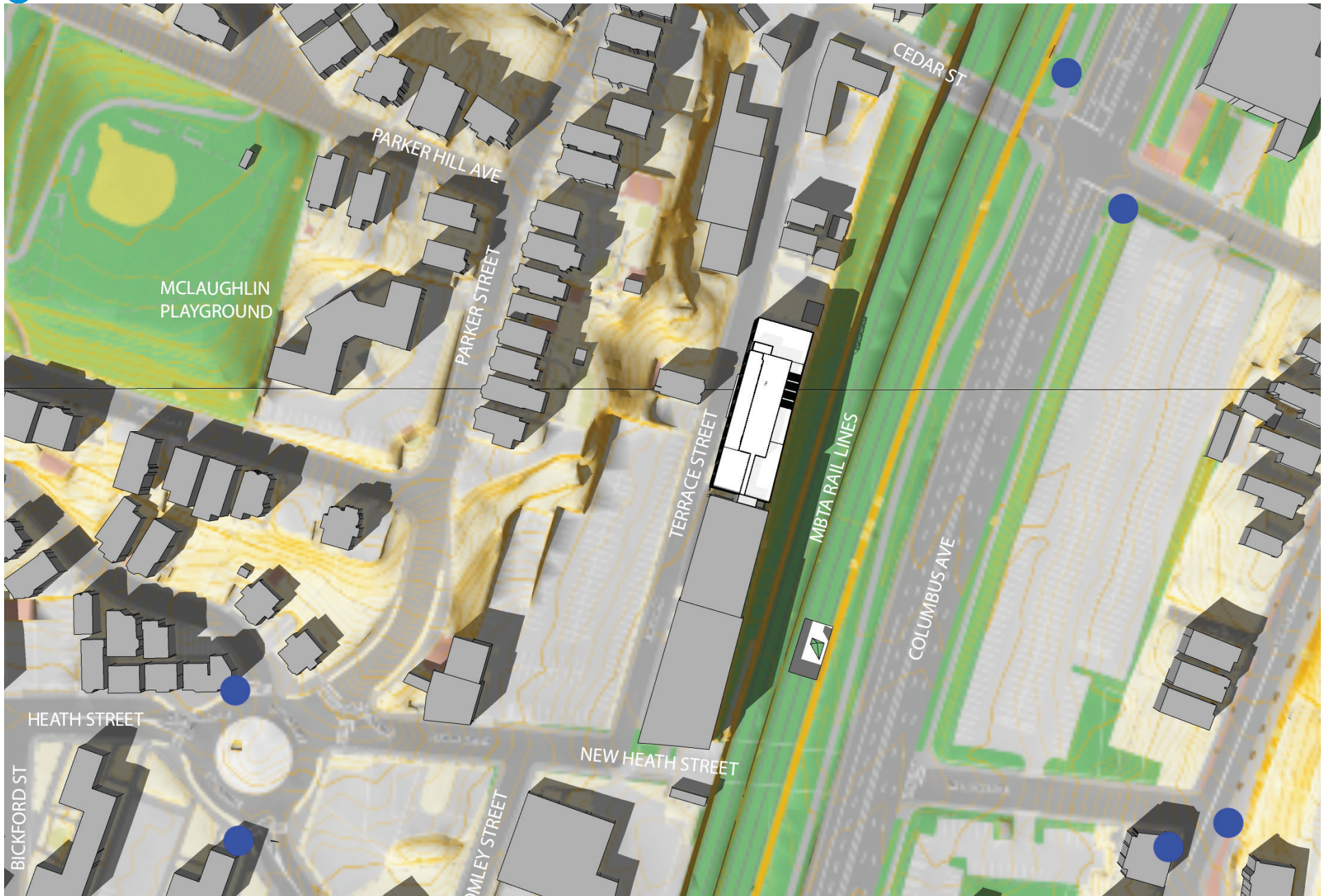
Figure 4.1-11 Shadow Study: September 21, 3pm Alt 37.5 Azimuth 227.2
