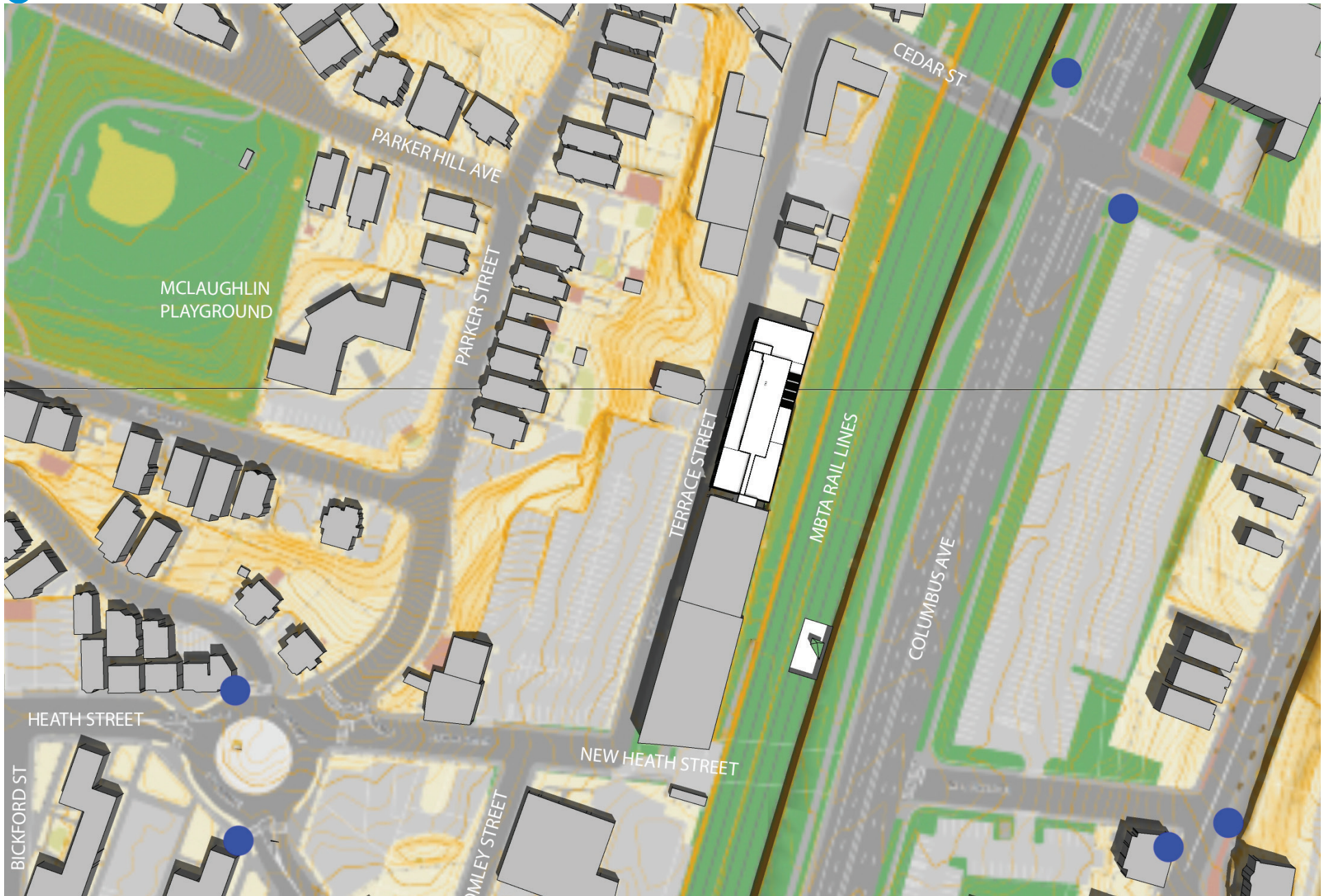
Figure 4.1-6 Shadow Study: June 21, 12pm Alt 68.8 Azimuth 149.5
