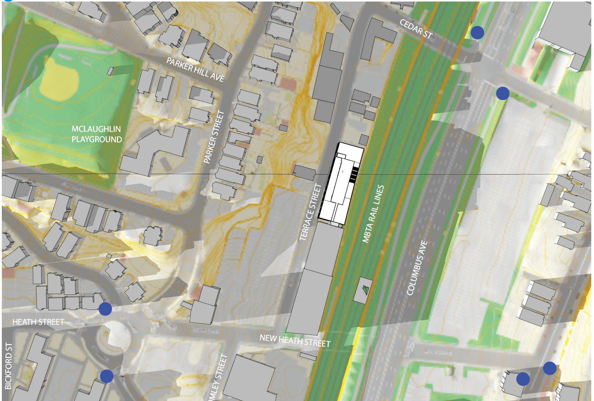
Figure 4.1-4 Shadow Study: March 21, 6pm Alt 9.8 Azimuth 261.5
