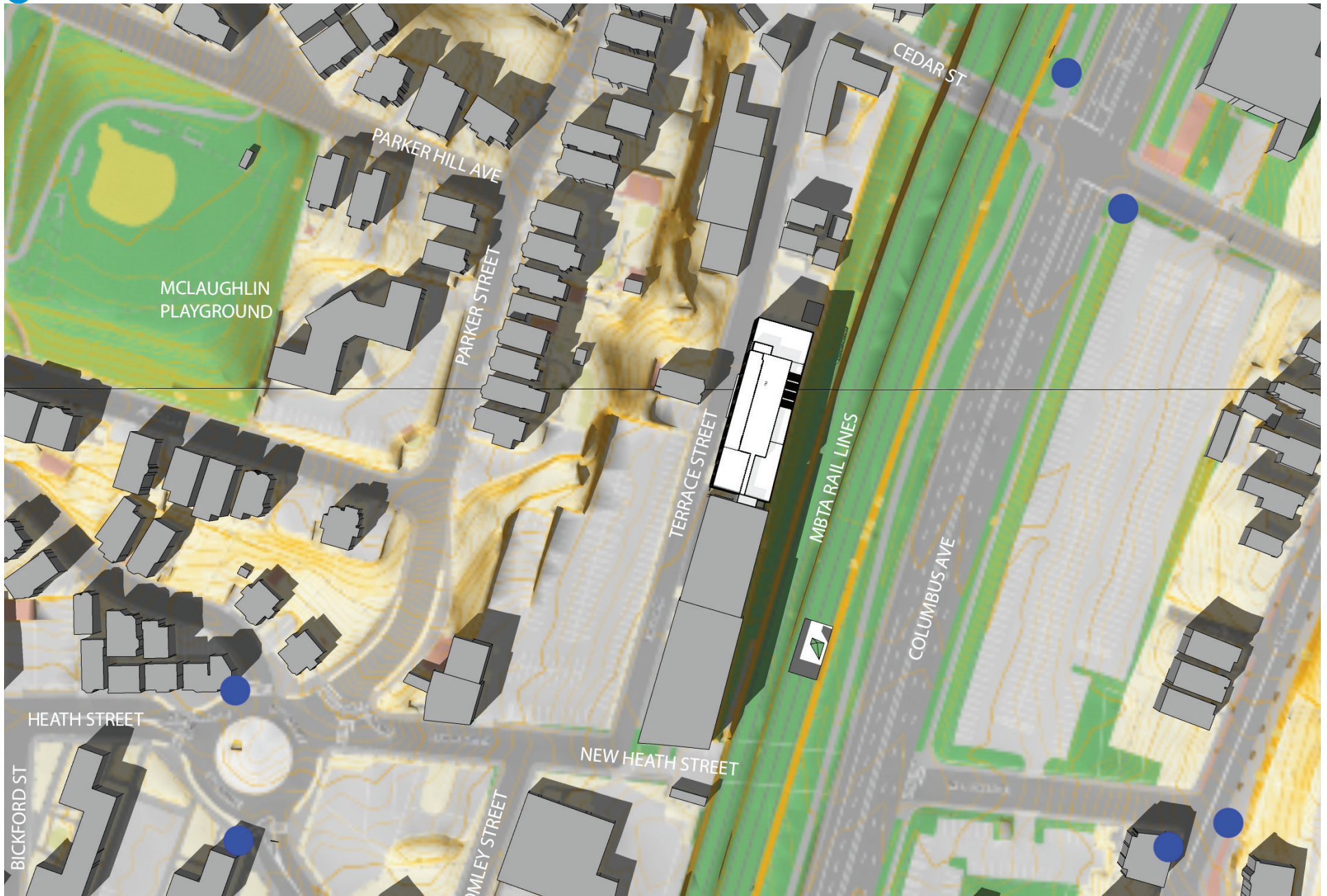
Figure 4.1-3 Shadow Study: March 21, 3pm Alt 39.1 Azimuth 223.2
