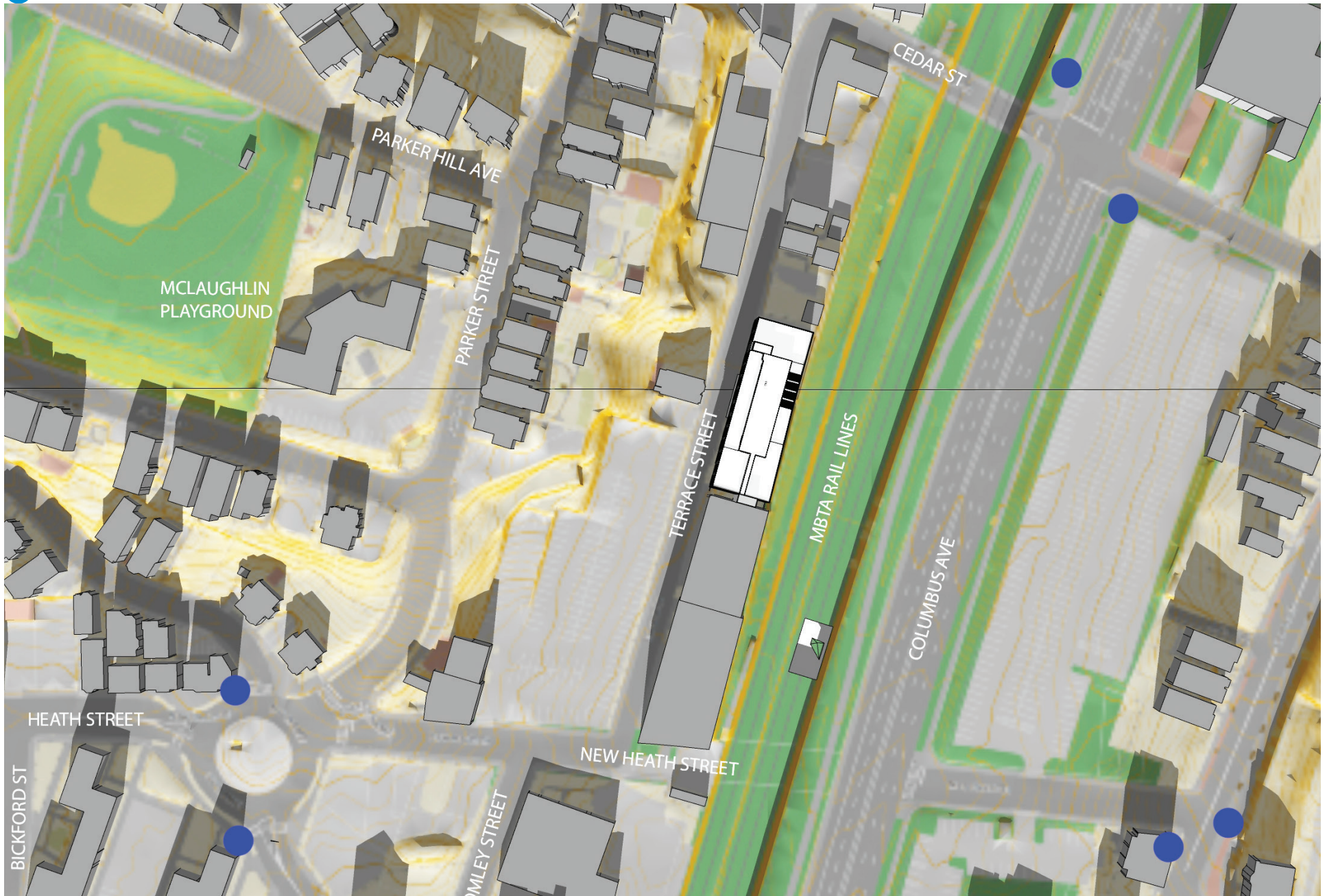
Figure 4.1-14 Shadow Study: December 21, 12pm Alt 24.2 Azimuth 184.4
