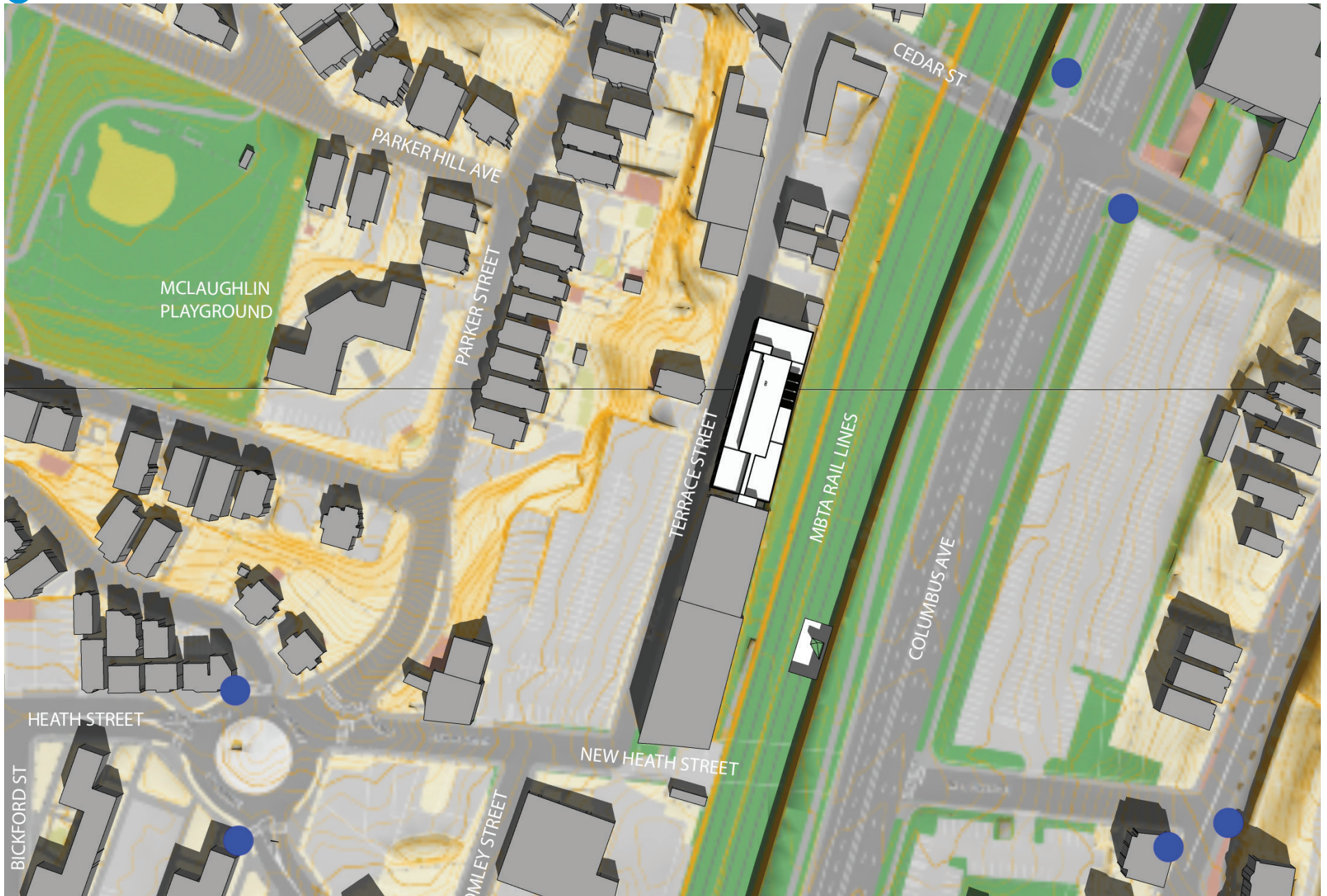
Figure 4.1-10 Shadow Study: September 21, 12pm Alt 47.5 Azimuth 166.1
