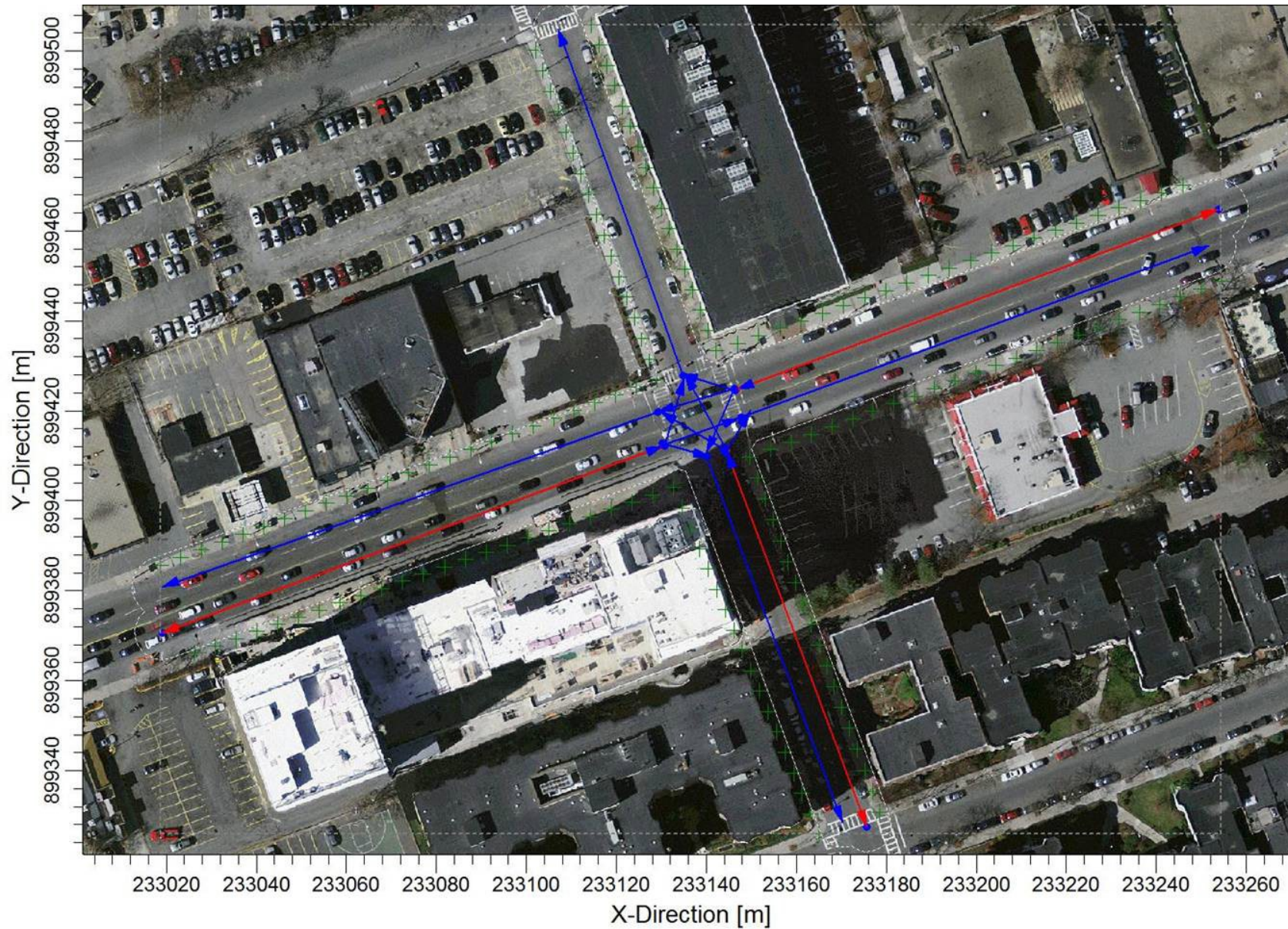
Figure 3.5-2 Link and Receptor Locations for CAL3QHC Modeling of Intersection of Boylston St. & Yawkey Way
