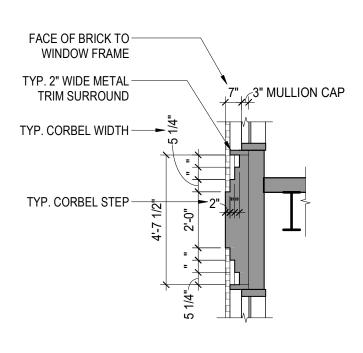
SECTION: TYP. MASONRY SLAB COVER
