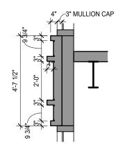
SECTION - TYP. METAL SLAB COVER
