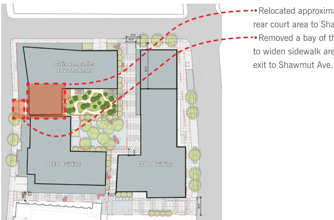
• Relocated approximately 22,000 sf from rear court area to Shawmut Ave. frontage • Removed a bay of the existing building to widen sidewalk area at garage entry/
