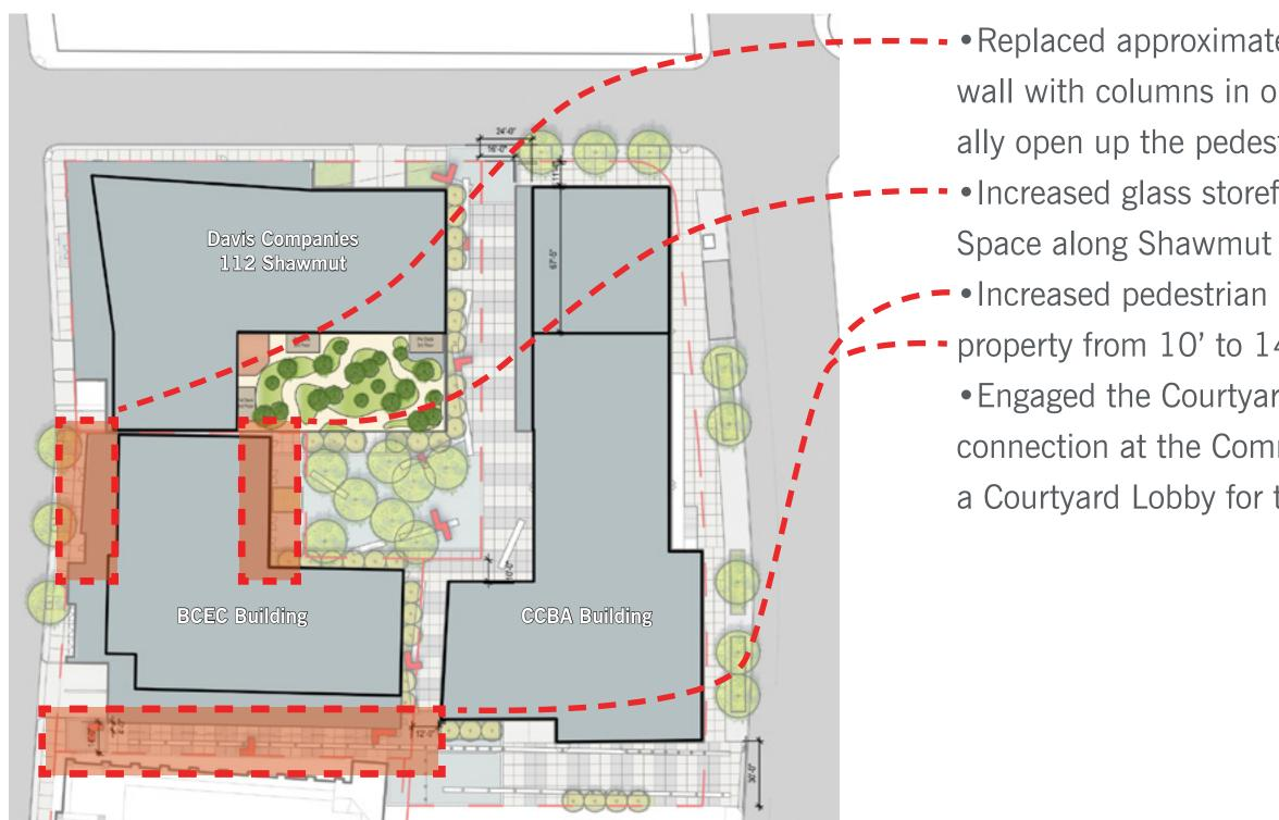
• Replaced approximately 50 linear feet of wall with columns in order to further visually open up the pedestrian way
