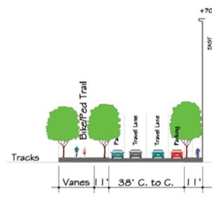
*Figure 137.* Western Edge Road along the Tracks (Service Road) Conceptual R.O.W. Section
