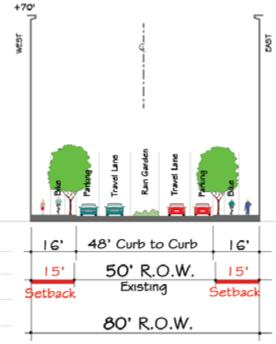
*Figure 130. D Street Conceptual R.O.W. Section*
