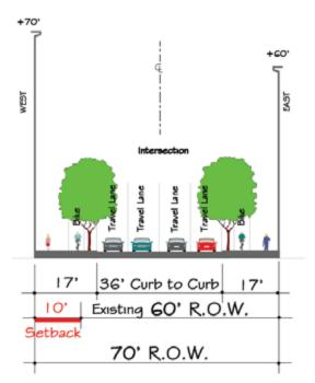
*Figure 136. Boston Street Conceptual R.O.W. Section*
