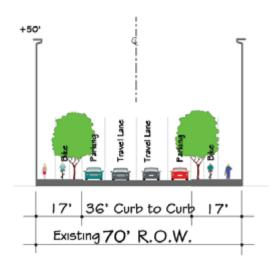
*Figure 138. Preble Street Conceptual R.O.W. Section*
