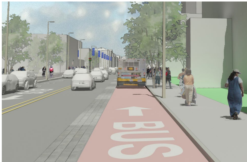
Figure 62. Conceptual drawing of potential "Complete Streets" improvements for Columbus Avenue, including landscaping, bus rapid transit (BRT) elements, protected bicycle accommodations, and improved sidewalks
