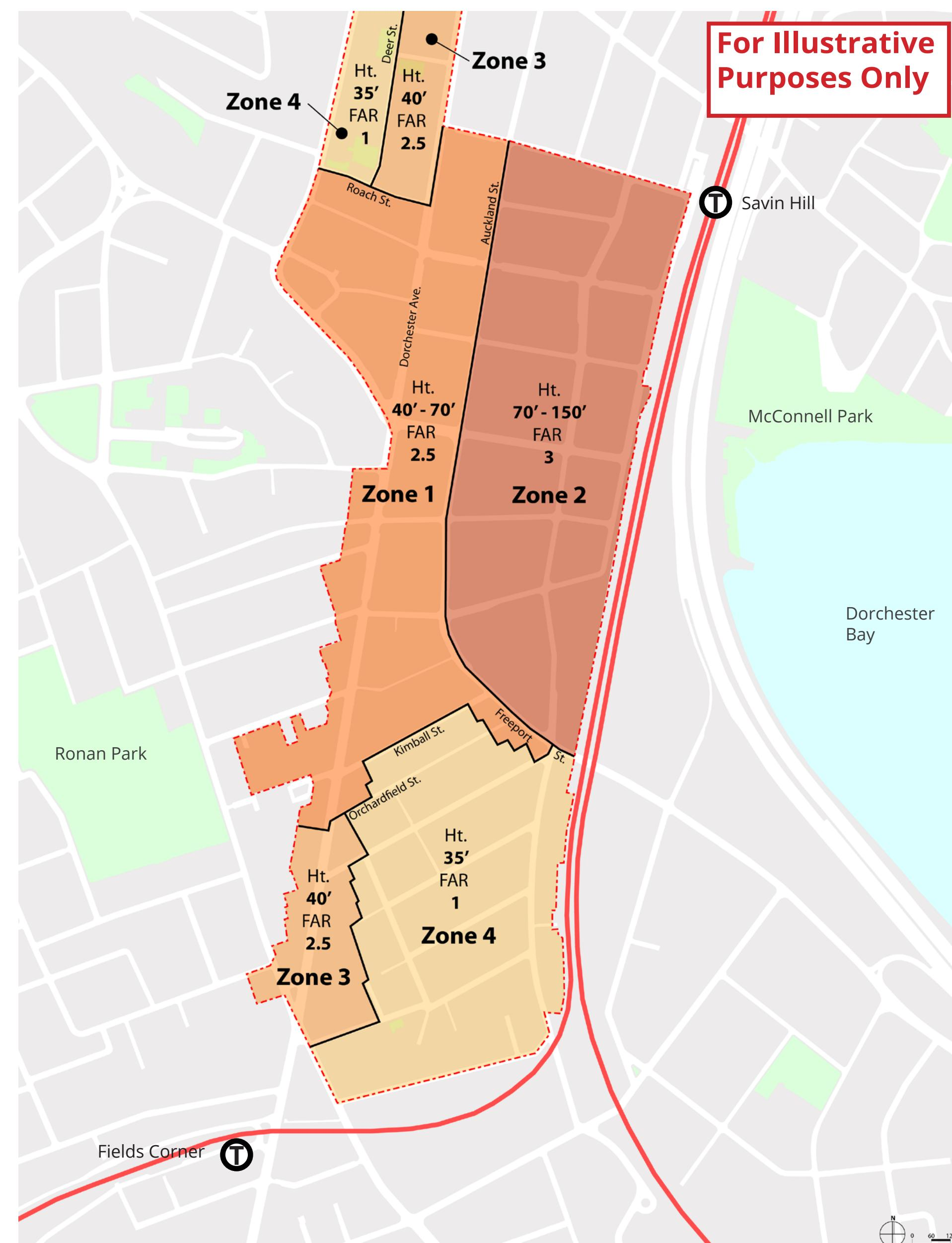
Height and floor area ratio diagram
