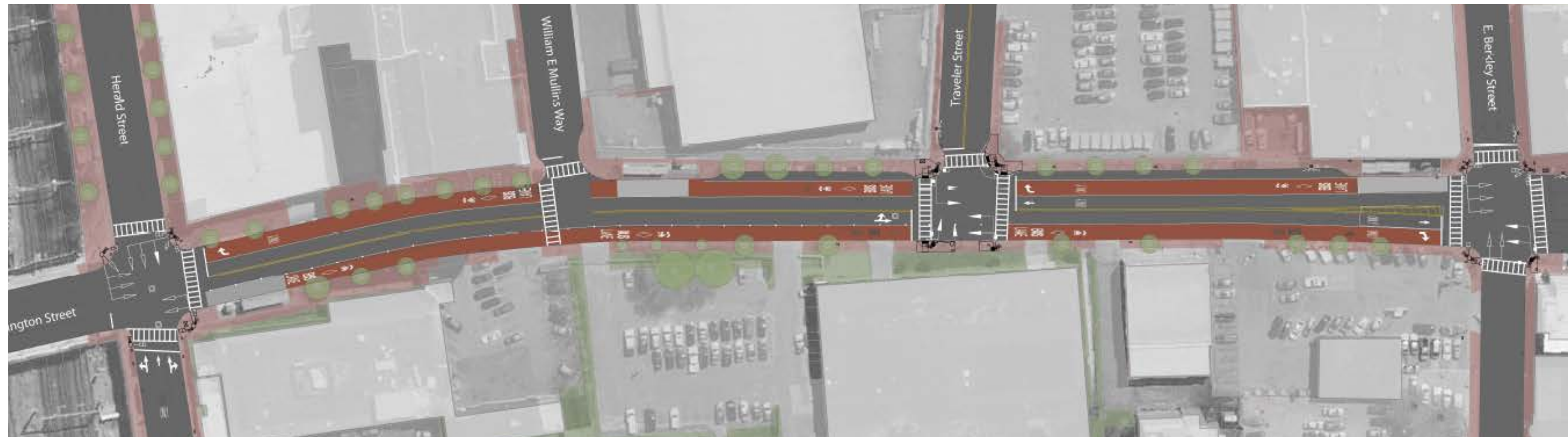
Washington Street – Design Changes for 2-way Operations Between Herald St. and E. Berkeley St.
