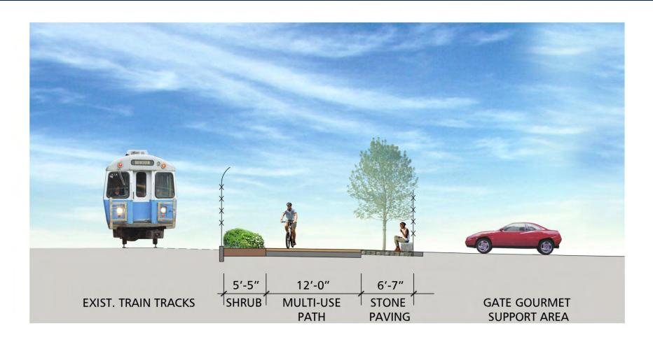
MULTI-USE PATH AT THE BACK OF GATE GOURMET SUPPORT AREA CROSS SECTION
