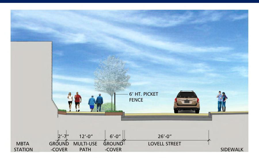
MULTI-USE PATH IN FRONT OF MBTA STATION CROSS SECTION
