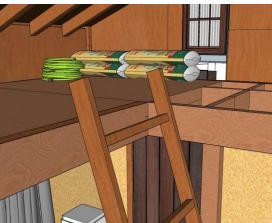
The roof has been designed to extend past the front door to provide protection from the elements for farmers and visitors to the site. The extended roof on the side also provides protection for both the shed itself as well as extra areas for storage/work.
